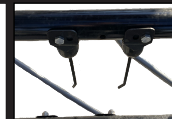
RAKE TEETH SPACING INCREASED FOR MORE STRIPPER BAR CLEARANCE
